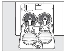
Replace the drain filters correctly (on the right and left) and tighten them securely.
