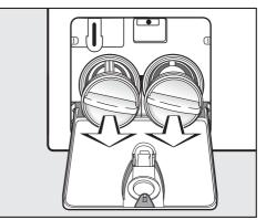
Remove the drain filters completely.
