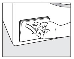
Open the drain pump access panel.
